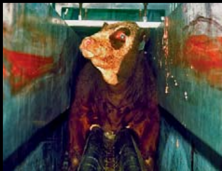
This photo by Dr. Temple Grandin shows a conveyor system commonly used to restrain cows and pigs during stunning.
